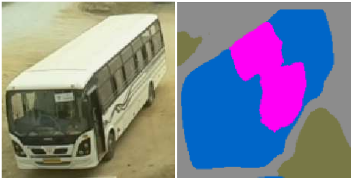
(a) Bounding box obtained after applying yolo (b) Segmented Output without class imbalance
